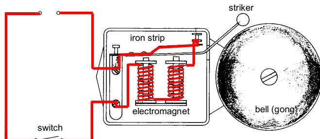
The coil is an electromagnet. It produces a magnetic field while a current passes through it.
