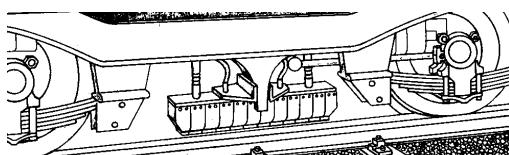
Streetcars have additional brakes using electromagnets (see picture).
