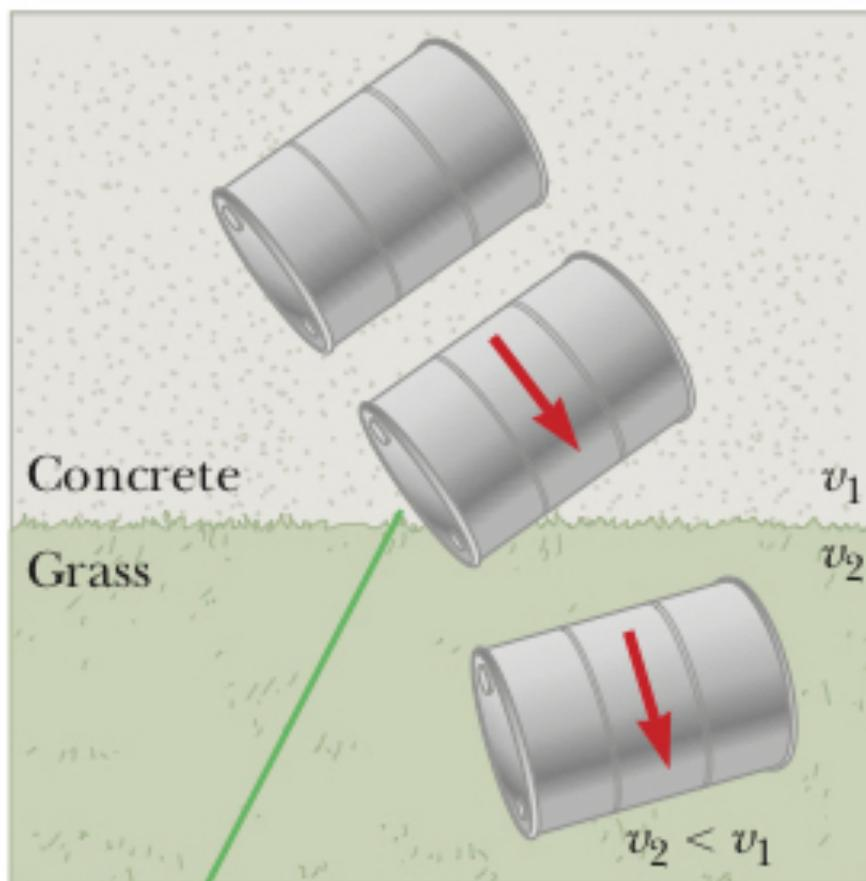
This end slows first; as a result, the barrel turns.
