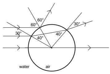
Bottom light ray: continues in a straight line, is not refracted as the angle between the normal and the light ray is 0
