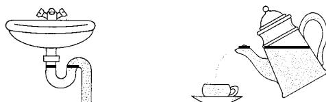
b) The U-shaped part is always filled with water, preventing bad smells from sewage from entering the house.
