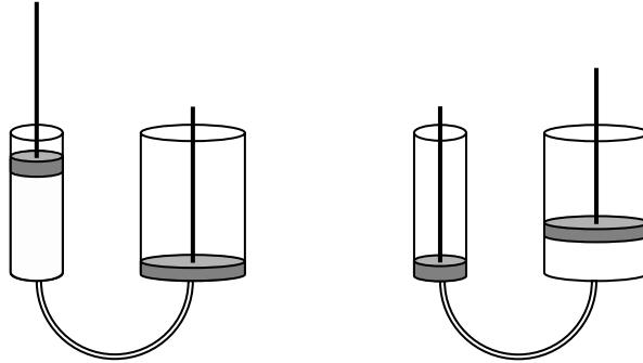
The volume of the liquid remains the same. Therefore the piston on the right doesn't rise as high as on the left side.
