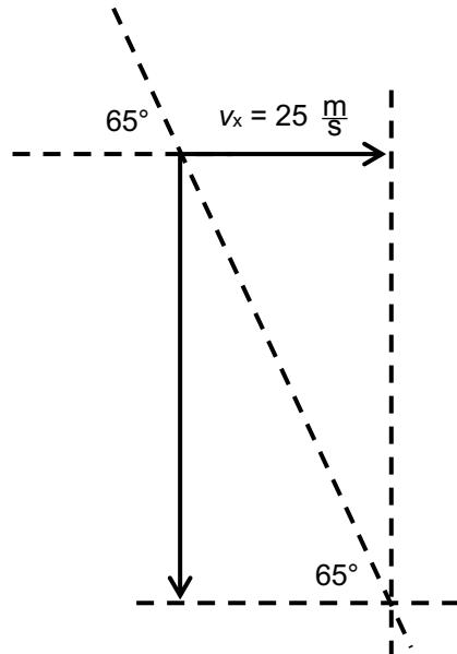
$$(\text{rechnerisch: } \tan(65^\circ) = 2.14 = \frac{v_y}{v_x} \Rightarrow v_y = 2.14 \cdot v_x = 2.14 \cdot 25 \frac{\text{m}}{\text{s}} = 53.6 \frac{\text{m}}{\text{s}})$$
