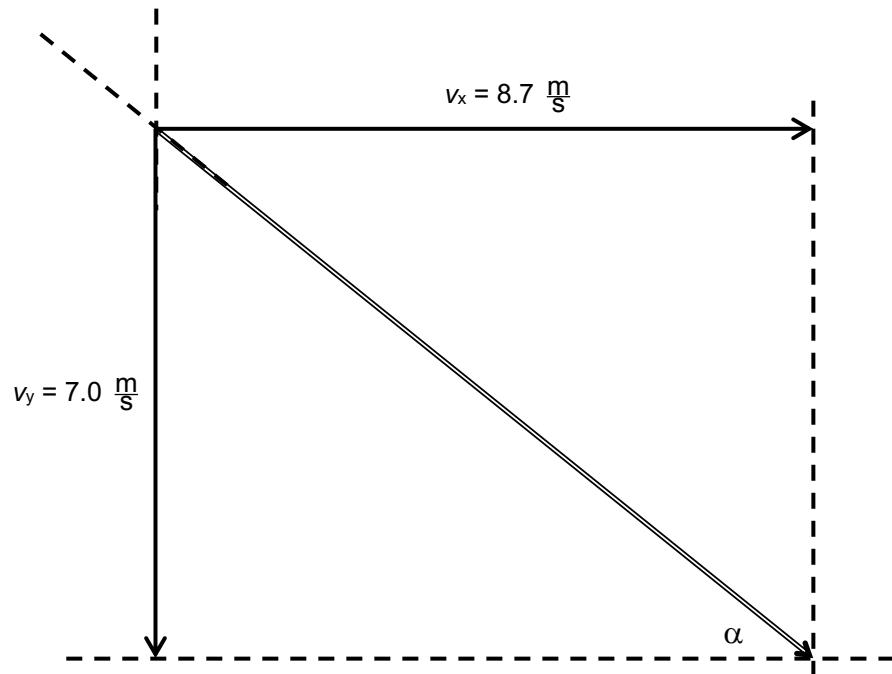
$$(\text{rechnerisch: } \tan \alpha = \frac{v_y}{v_x} = \frac{7.0 \frac{\text{m}}{\text{s}}}{8.7 \frac{\text{m}}{\text{s}}} = 0.8046 \quad \Rightarrow \quad \alpha = \arctan (0.8046) = \underline{\underline{39^\circ}})$$
