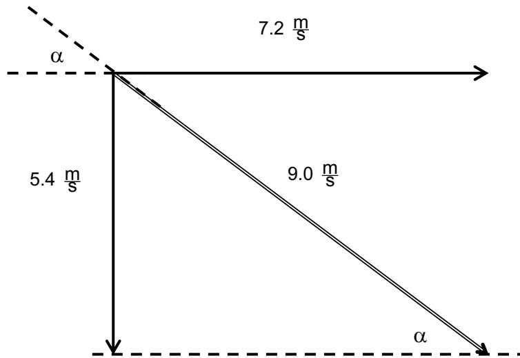
$$(\text{rechnerisch: } \frac{v_y}{v_x} = \tan \alpha = 0.75 \Rightarrow \alpha = \arctan(0.75) = \underline{\underline{37^\circ}})$$
