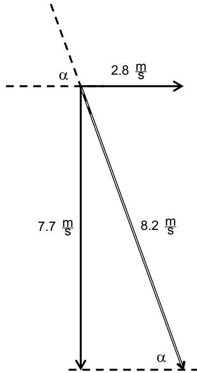
$$(\text{rechnerisch: } \frac{v_y}{v_x} = \tan \alpha = 2.75 \Rightarrow \alpha = \arctan(2.75) = \underline{\underline{70^\circ}})$$
